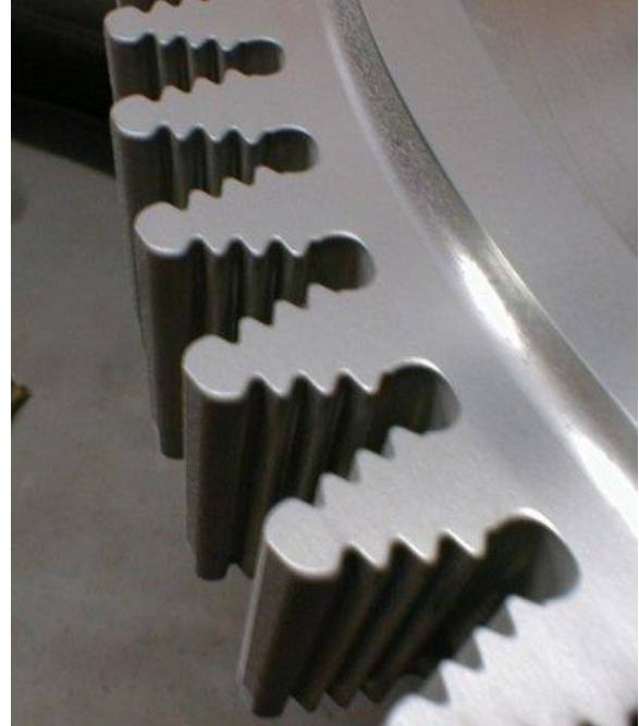
Figure 15 - Detail of turbine disc following a Turbo-Abrasive Machining and Finishing process. This automated dry process deburrs, edge-contours and develops isotropic surfaces simultaneously.
