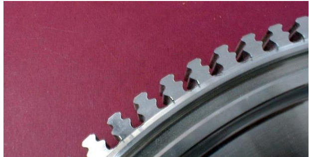
FIGURE 10 - BURR AND EDGE CONDITION PRIOR TO TAM PROCESSING
