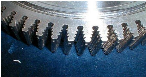
Figure 14 - Detail of turbine disc prior to Turbo-Abrasive Machining and Finishing.
