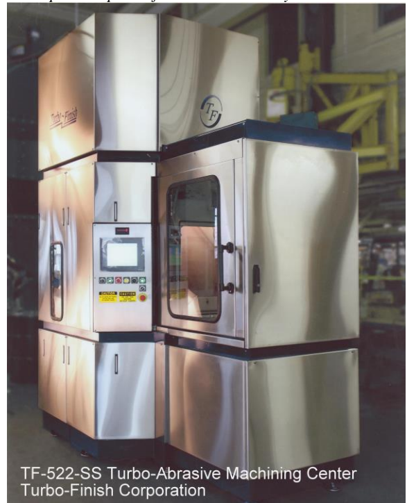
Figure 16 – The Turbo-Finish processes utilize high speed part rotation and abrasive fluidized bed technology to deburr and finish complex rotating shapes in a rapid dry-process horizontal spindle finish method. The automated method can reduce deburring cycle times from hours to minutes.
