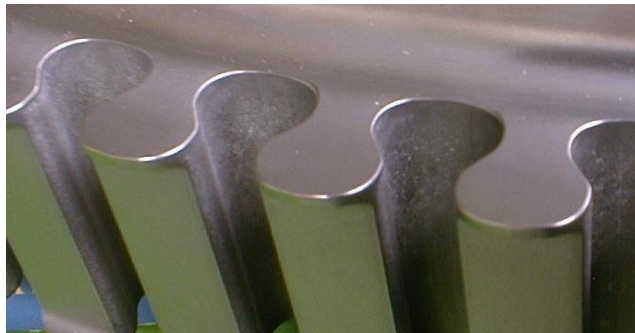
Figure 4 - After TAM Processing, sharp edges have been replaced with polished edge contoured. Two TAM processes with sequentially finer abrasive material were used.
