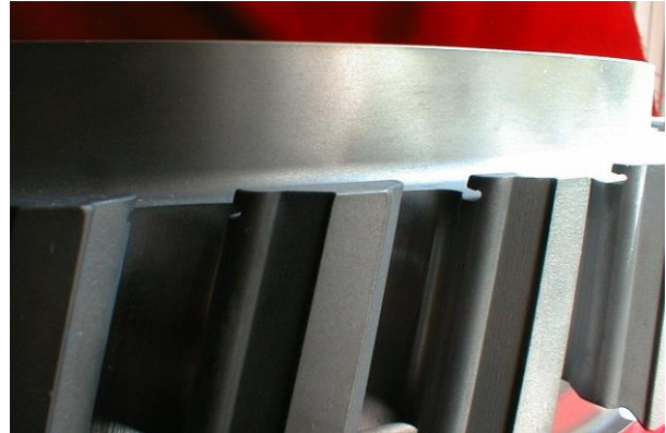
Figure 6 - Turbo-Abrasive Machining processes make it possible to edge contour and surface finish part features and geometries not accessible by other finishing methods. This ability is facilitated by both the relatively small size of the abrasive media and the high pressure nature of the part surface and media interaction.
