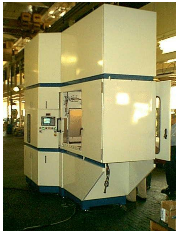
Figure 1 - Model Tf-522 Turbo-Abrasive Machining Center For Deburring And Edge Contouring Turbine Disks Up To 500mm In Diameter.
