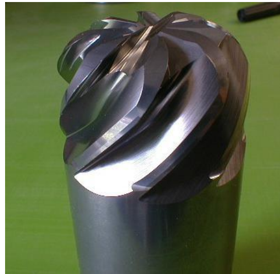
Figure 7 - Edge-finishing with mass finishing methods can improve speed and feed performance and service life of cutting tools (Photo credit: D. A. Davidson, SME MMR Tech Community)
