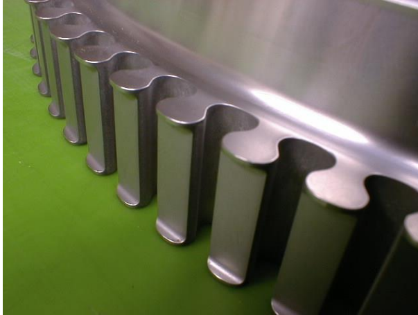
Figure 4 – Aerospace rotating hardware edge and surface finished with Turbo-Abrasive Machining (TAM). (Photo credit: Dr. Michael Massarsky, Turbo-Finish Corporation)
