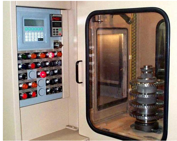
Figure 5 – Rotating aerospace hardware can be rapidly edge and surface finished using a high-speed, dry, horizontal spindle finishing method known as TAM (Turbo-Abrasive Machining) Photo credit: Dr. Michael Massarsky, Turbo-Finish Corporation
